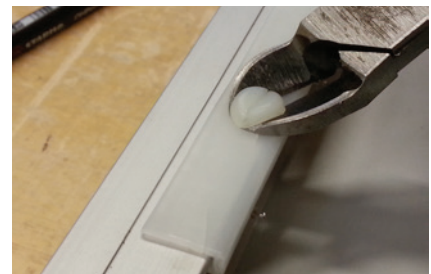
Cut off screw head
