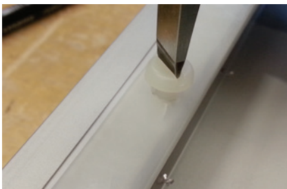
Refit guide, fit screw
